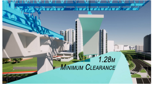
Fig. 5. Quantitative Assessment of Minimum Clearance with Adjacent Facilities during Equipment Operation through VR Simulation
