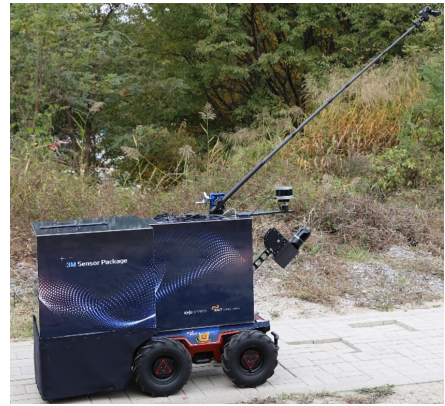
Fig. 2. Unmanned Ground Vehicle Developed for Ground Monitoring Purpose
